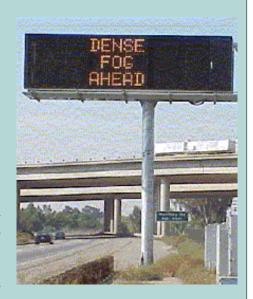
**Intelligent Transportation Systems (ITS),** a major focus of the last decade, seek to take existing detection, computer, and communication technologies and apply in them in an integrated way to increase the safety and efficacy of road transportation. For example, in Minneapolis-St. Paul, real-time data from freeway traffic counters are input into freeway capacity algorithms which, in turn, automatically regulate traffic lights at entry ramps to improve traffic flow.
