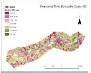
Elevation differences between the USGS National Elevation Dataset and lidar data, Swannanoa River, North Carolina. Areas in red and pink are lower than appear on FEMA flood maps and suggest that the floodplain extends further than expected. SOURCE: Courtesy of T. Langan, North Carolina Floodplain Mapping Program, used with permission.
