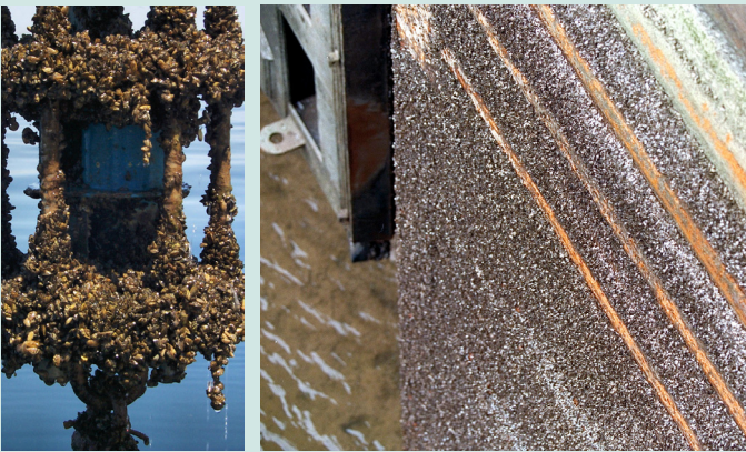
Zebra mussels cover a current meter in Lake Michigan (left) and infest the walls of a lock on the Arkansas River (right).
