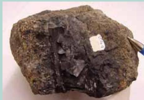
**Figure 1.** A sample of the uranium-containing mineral uraninite.
