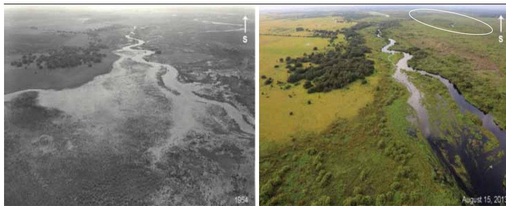
Figure 1. Photos showing the natural historic Kissimmee River and floodplain in 1954 prior to channelization of the river (left), and the same view after canal filling and river restoration (right). The filled channel is circled in the right-hand figure. SOURCE: T. Morgan, SFWMD, personal communication, 2013.
