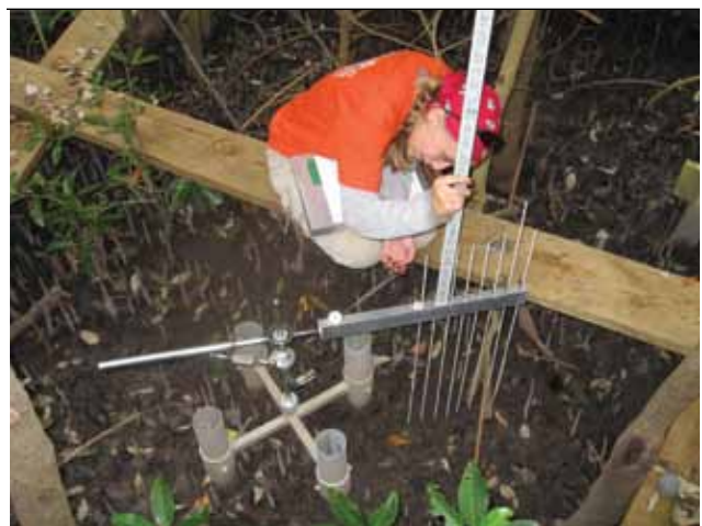
Figure 3. A sediment elevation table (SET) is used to measure short-term changes in the elevation of the soil surface in an Everglades mangrove forest to better understand the rate of peat accretion or subsidence. Source: USGS.
