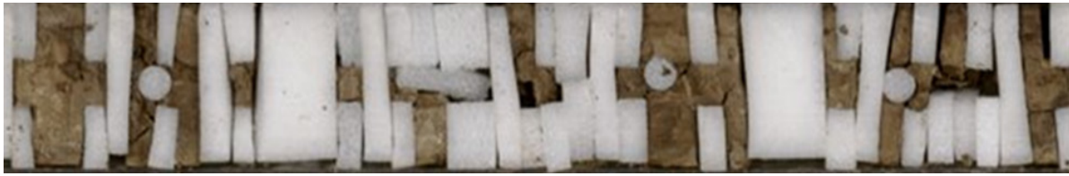
FIGURE 1: Example of a highly sampled core for an interval of high scientific interest. Styrofoam spacers (white) replace samples that have already been used. SOURCE: JRSO
