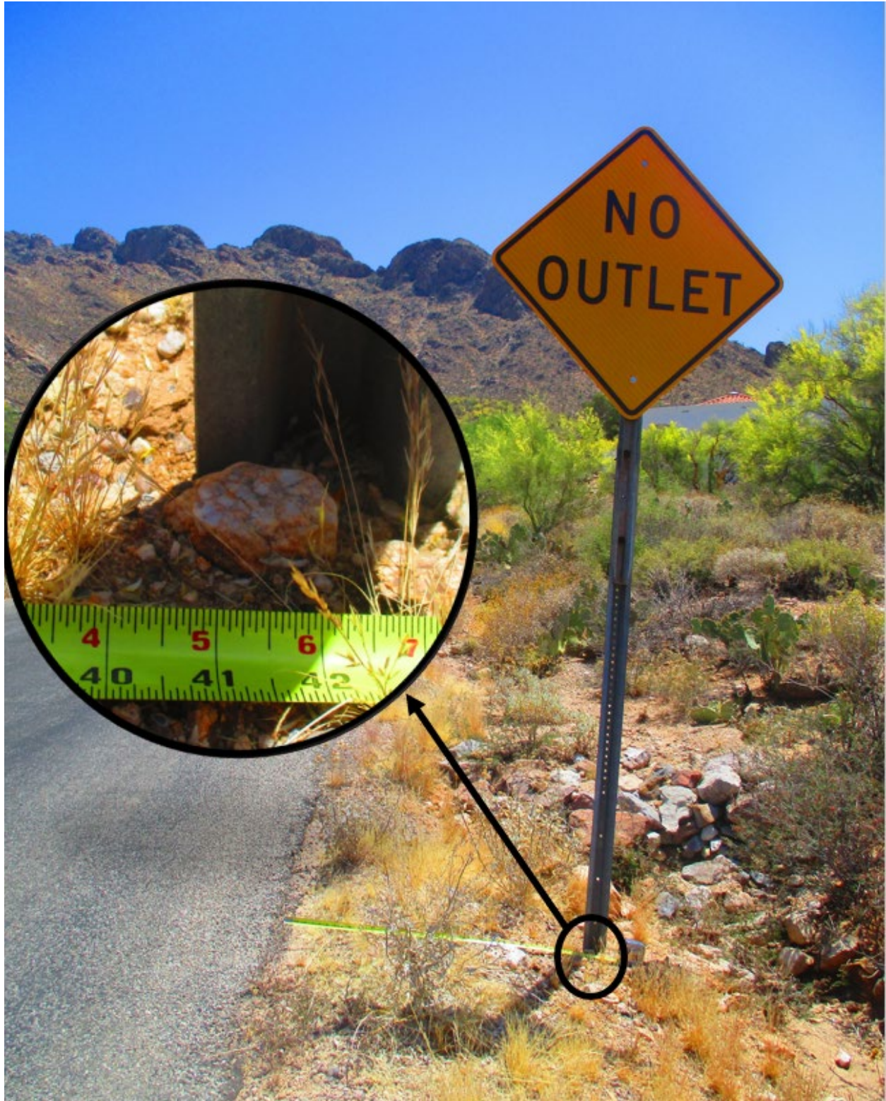
Figure 6. Offset measurement of sign support, this offset is 3.4 feet (41 inches).
