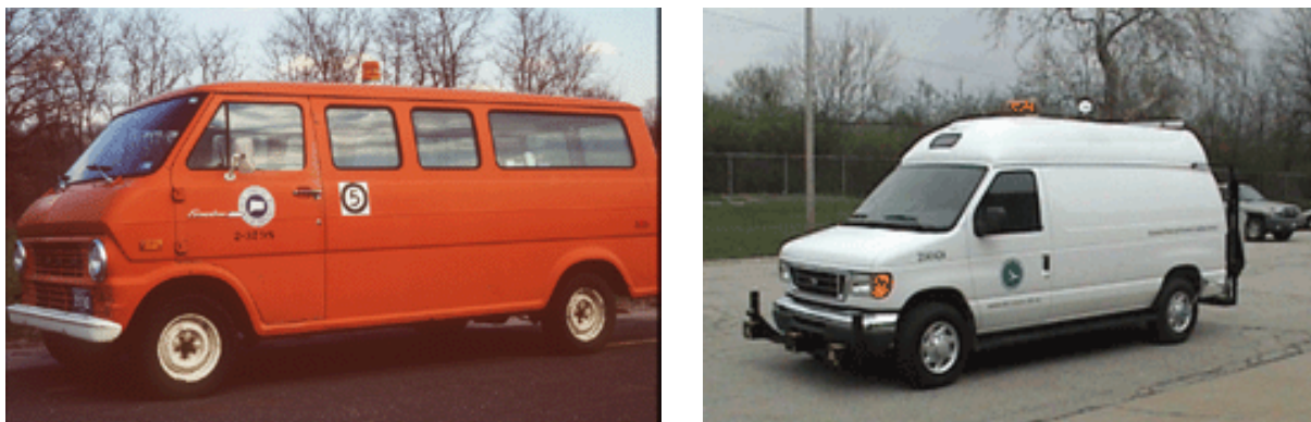
Figure 19. The first imaging van used by Connecticut DOT (left) and the current imaging van used by Ohio DOT. [36, 37]
